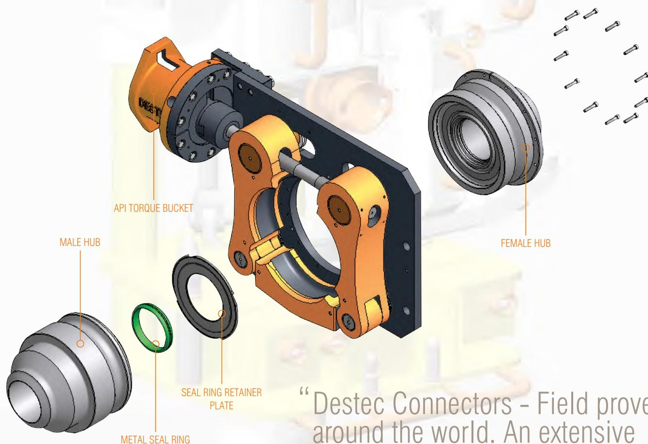
“Destec Connectors - Field proven around the world. An extensive track record subsea with many years of service”
