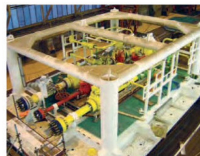
Desflex Compact Flanges are used extensively on sub-sea manifolds
